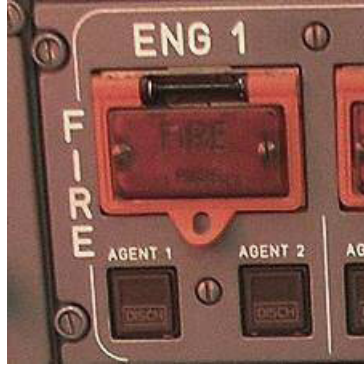
Fig. 3: Engine 1 FIRE push-button on the overhead panel.
